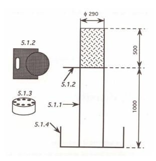
Figure 1. Equipment for determination of the bulk volume of a chip sample:
