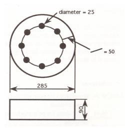
Figure 2. Wooden lid (5.1.3), perforated with eight holes, dimensions in millimetres.
