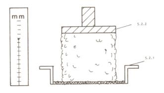
Figure 1. Determination of specific volume 5.2.1 Dish with perforated bottom 5.2.2 Load, 500 g
