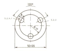
Figure 5. Mounting of the electrodes in the load
