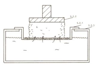
Figure 2. Determination of absorption time 5.2.1 Dish with perforated bottom 5.2.2 Load, 500 g 5.2.3 Container for water
