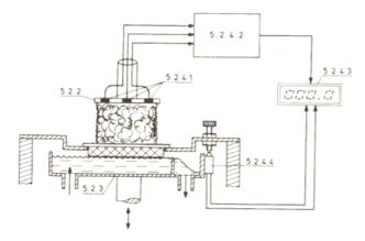
*Figure 4. Apparatus for determining the absorption time*
