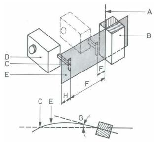
Figure. Principle of the bending resistance tester.
