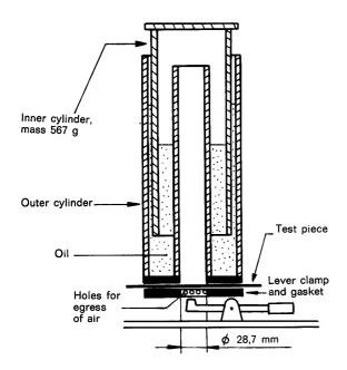
Figure 1. Diagram of the Gurley apparatus (not to scale).
