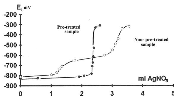
*Figure 1.* Titration curves for pre-treated sample and non-pre-treated sample. If the non-pre-treated sample gives two inflection points, the result must be rejected and pre-treatment must be done before a new titration is carried out.
