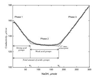
Figure 1. Determination of the total amount of charged groups in a CTMP by conductoimetric titration.
