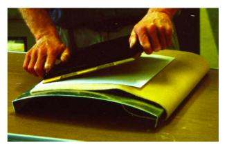
Figure 1. A couching system comprising a curved plate covered with a felt.
